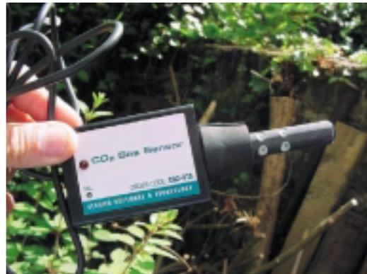
*A carbon dioxide gas sensor - useful in the laboratory and in the field - for taking direct measurements of carbon dioxide concentration*
